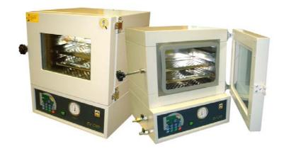
The EV 018 vacuum oven has the ideal design for gentle drying of heat labile samples and experiments under inert gases and optimizes under inert gases and optimises the control of temperature and pressure is obtained by the sheet heaters surrounding the chamber with the combination of PID microprocessor control system.
