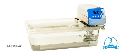
Clifton NE4D/CT digital stirred baths come complete with sturdy clear polycarbonate tank, allowing observation of samples. Complete with stainless steel shelf designed for good water circulation and temperature uniformity. All Clifton stirred baths feature a low liquid level float switch, which ensures heating is switched off if the liquid falls below the recommended level.
