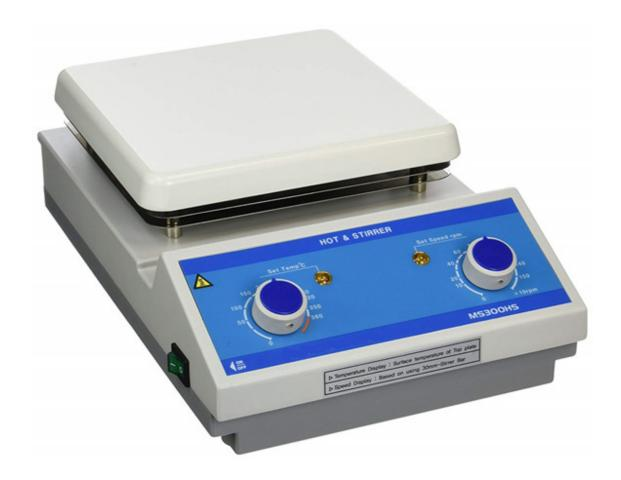
The MS-300 230V 680W Hot Plate Stirrer offers a large heating area of  $180 \times 180$ mm and is ideal for use with flat-bottomed vessels. With controlled heating up to  $400^{\circ}C$ . The speed of the built-in magnetic stirrer can be controlled between 100 and 1500rpm.
