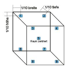
Positions of probes according to NF X15-140
