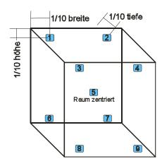
Positions of probes according to NF X15-140
