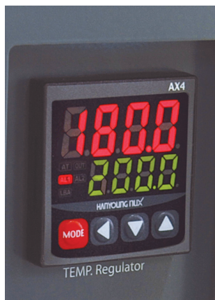
Individual over temperature limiter
