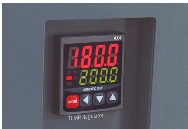
Individual over temperature limiter
