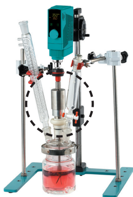
Application of magnetic drive
