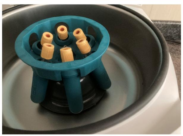
**Incorrect loading:** ALL the following are out of balance so will trigger the sensor:
